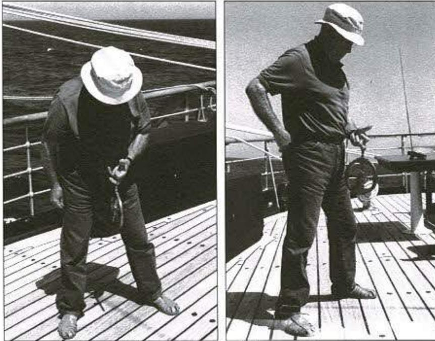
The plane of the instrument should be in the vertical plane of the sun.
